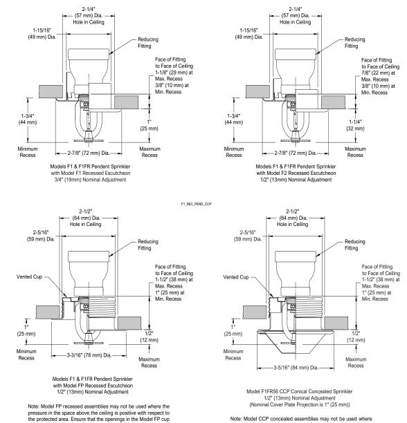
Note: Model CCP concealed assemblies may not be used where the pressure in the space above the ceiling is positive with respect to the protected area. Ensure that the openings in the Model CCP cup are unobstructed following installation.
