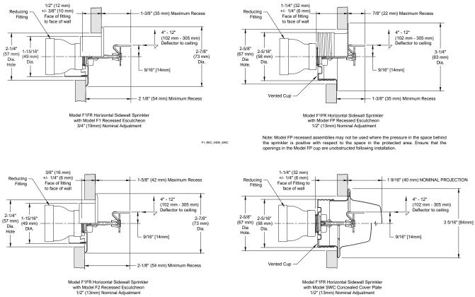
Note: Model SWC concealed assemblies may not be used where the pressure in the space behind the sprinkler is positive with respect to the space in the protected area. Ensure that the openings in the Model SWC cup are unobstructed following installation.
