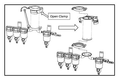
4) Remove the old Cartridge(s) & Spacer from the Module(s) by <u>PUSHING</u> a new Cartridge into each Module, and in the process ejecting each old Cartridge(s) & the Spacer. Then reinsert the Spacer in the 10" Module on the same side as the Cartridge's alignment pins. Note that <u>only</u> the 10" Module has a Spacer, the 8" Expansion Modules only have a Cartridge, see adjacent figure.
