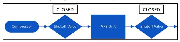
2) Depressurize the VPS unit to atmosphere (0 PSIG) by slowly opening the Drain Port on any filter. This can be accomplished by rotating the Knob at the very bottom of any filter Clockwise to the position marked "O". Do not disengage the bowl from any filter or attempt to loosen any other fittings to depressurize the VPS unit.
