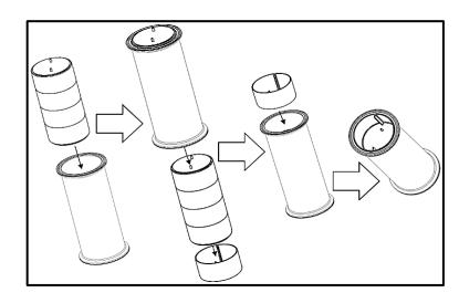
5) Dispose of the used Cartridge(s) & Gaskets by conventional means, in accordance with state and local guidelines if applicable. Save the Spacer, and store for later reuse, see adjacent figure.
